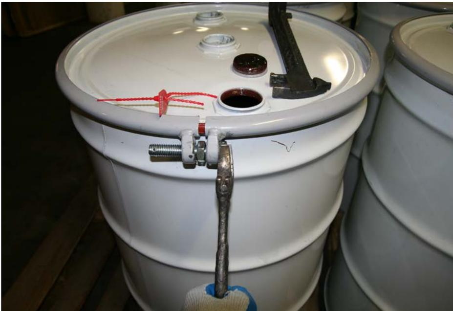
**Remove red drum tag/seal and loosen bolt. Do not remove until all pressure on container has been relieved.**
