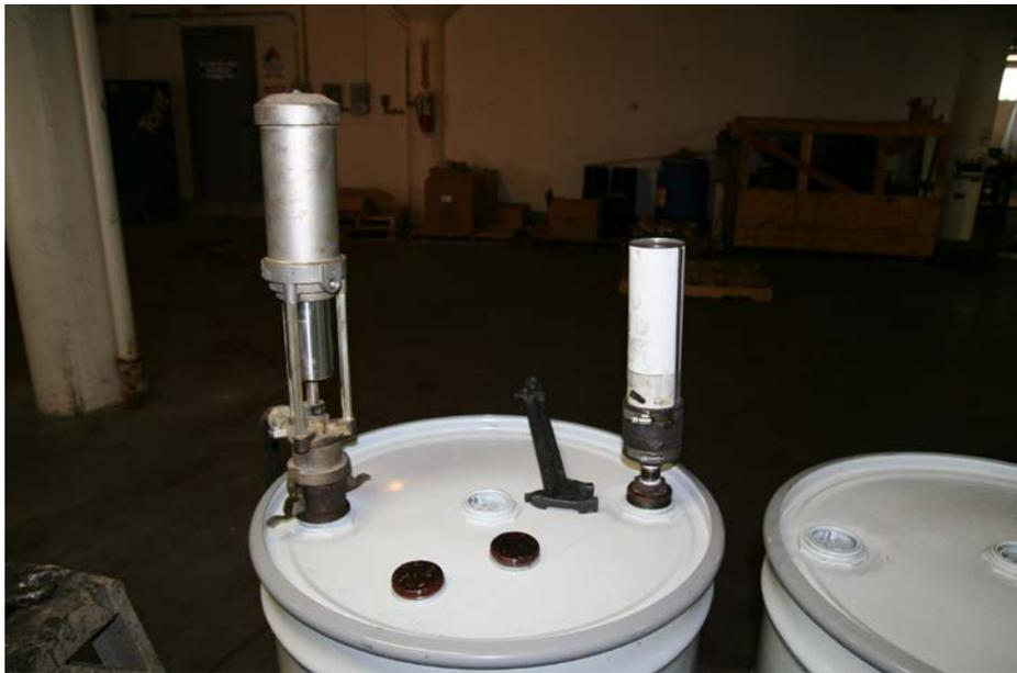
After mixing, replace lid and seal tightly. Use collars on drum pumps and use moisture dessicants on the isocyanate (Component "A") drum. Note: Picture shown above is the resin (Component "B") drum.
