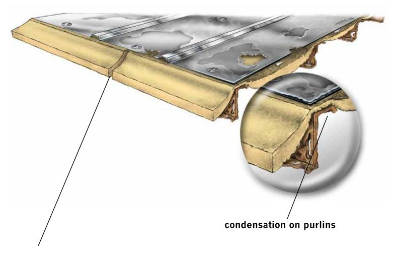
Air spaces and seams between fiberglass blanket insulation permit chemical and water vapors to infiltrate and condense on metal roof, causing corrosion and saturation of insulation. Compressed insulation above purlins causes condensation on purlins which accumulates in the lower flange, resulting in corrosion and structural failure.
