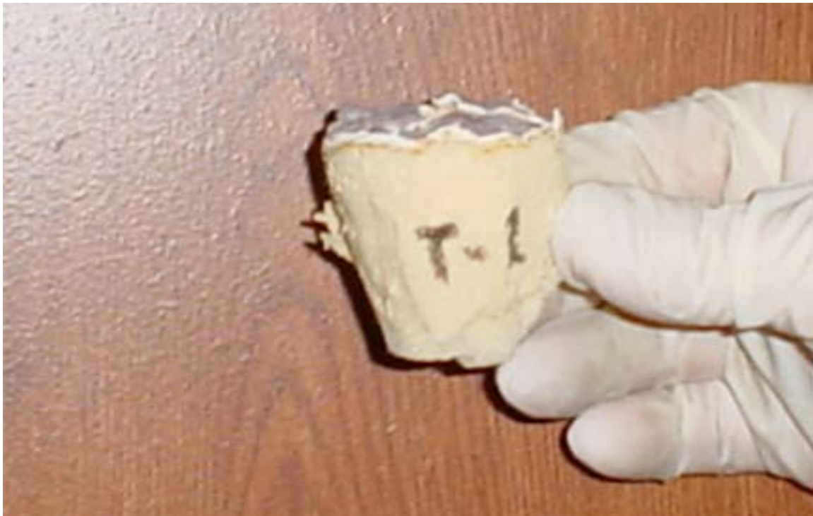
ILLUSTRATION 6: CROSS SECTION VIEW OF TEST CORE SAMPLE 1. THERE WAS NO VISIBLE MATERIAL DEGRADATION NOTED.
