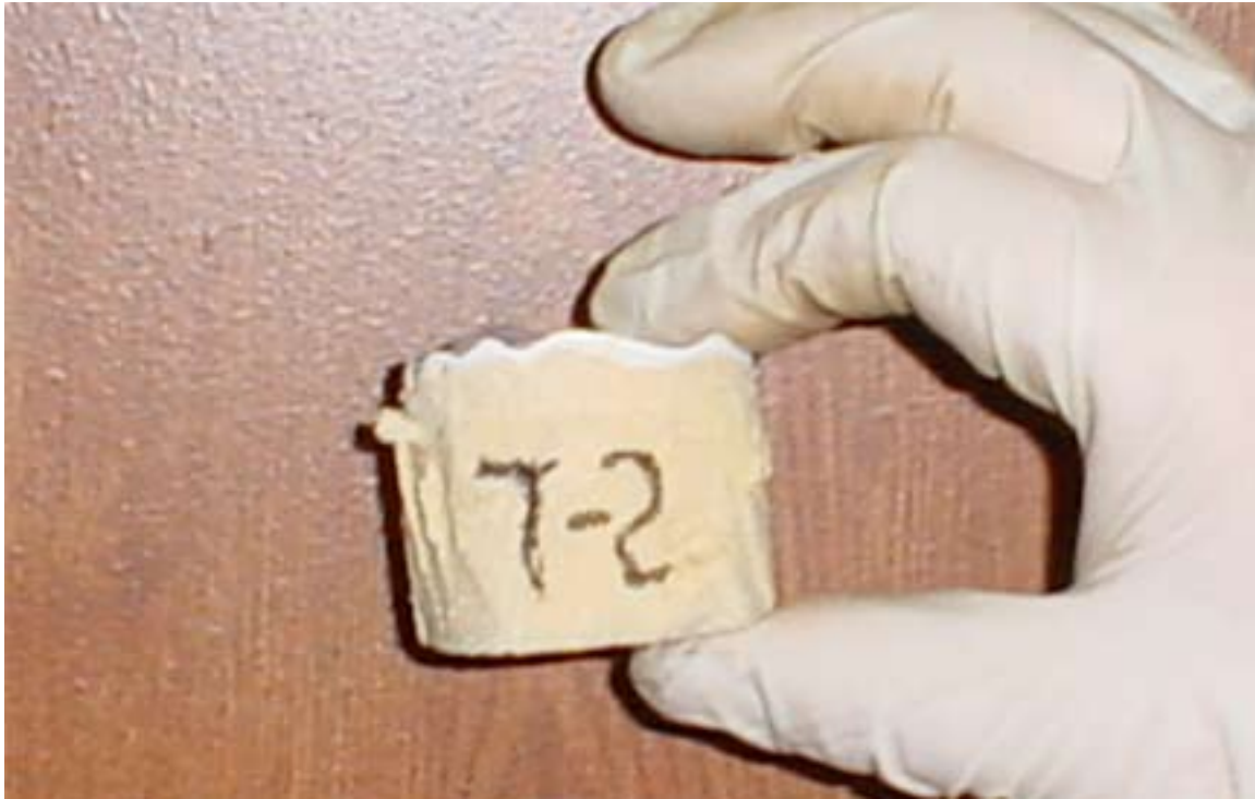
ILLUSTRATION 10: CROSS SECTION VIEW OF TEST CORE SAMPLE 2. THERE IS NO VISIBLE MATERIAL DEGRADATION NOTED.
