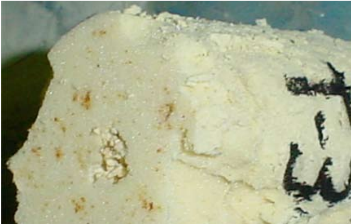
ILLUSTRATION 12: CROSS SECTION VIEW OF TEST CORE SAMPLE 3. THERE IS NO VISIBLE MATERIAL DEGRADATION NOTED.
